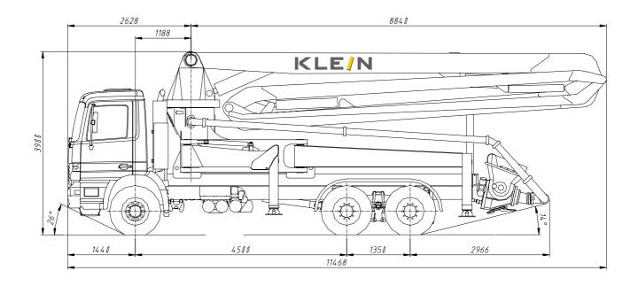
BOOM TYPE GROSS WEIGHT, INCL. TRUCK AND STANDARD PUMP UNIT
