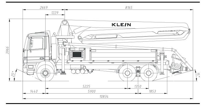
BOOM TYPE GROSS WEIGHT, INCL. TRUCK AND STANDARD PUMP UNIT
